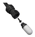
Rinse the filters, contrary to their suction direction, thoroughly. For this you can use a normal hosepipe with a connecting piece.
