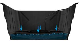
Put the filter coverplate (6) flush onto the filter sponge (8).
