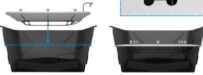
Squeeze the power cable of the circulation pump into the lowest hole of the sealing (18).
