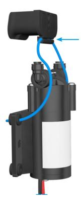
Now conjoin the 6mm hose (10) and the 8mm hose (11) with the connectors of the high pressure pump (2).
